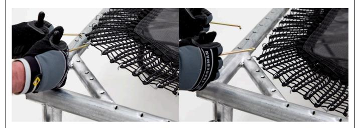
Please Note: In order to attach the hooks securely please use the provided tools and wear gloves to protect your hands. To make assembly easier we suggest that two adult persons attach the steel hooks at the same time on the opposite side using the same force and speed. To attach the corner hooks you may require 2 people using 2 sets of spring tools, attaching the hooks next to each other at the same time.
